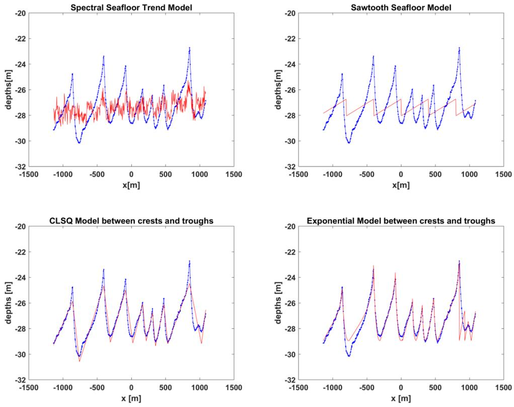
Figure 3: Additional alternative models; spectral, sawtooth, CLSQ between crests and troughs and exponential model between crests and troughs.
