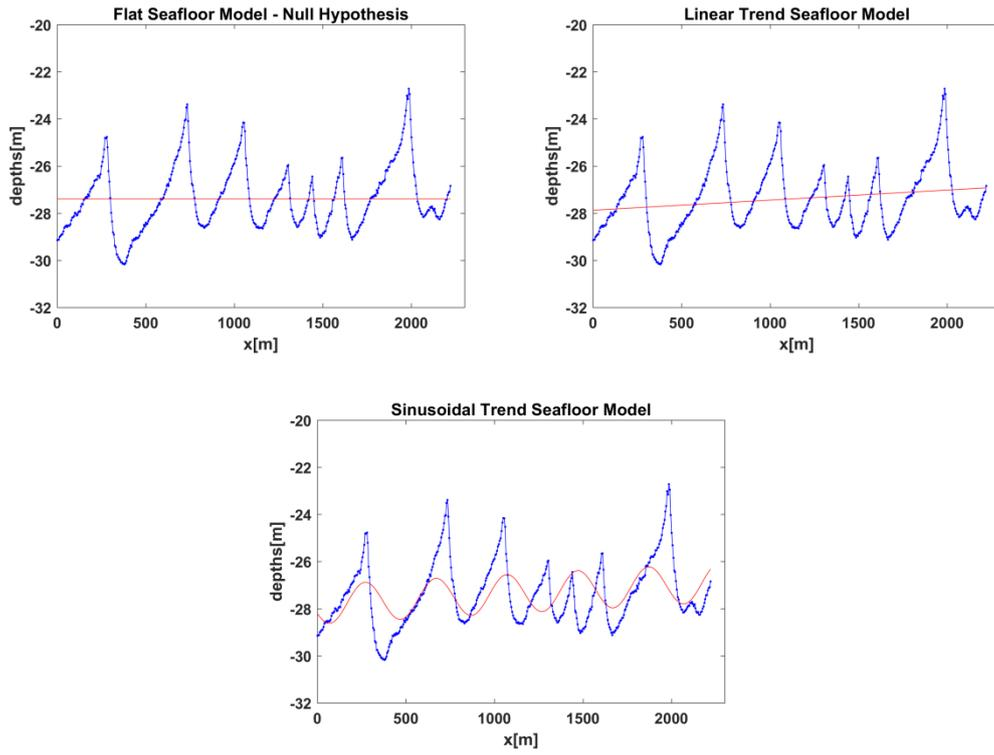
Figure 2: Blue line shows depth cross section of observations. Red line shows the stable, linear trend and sinusoidal model.
