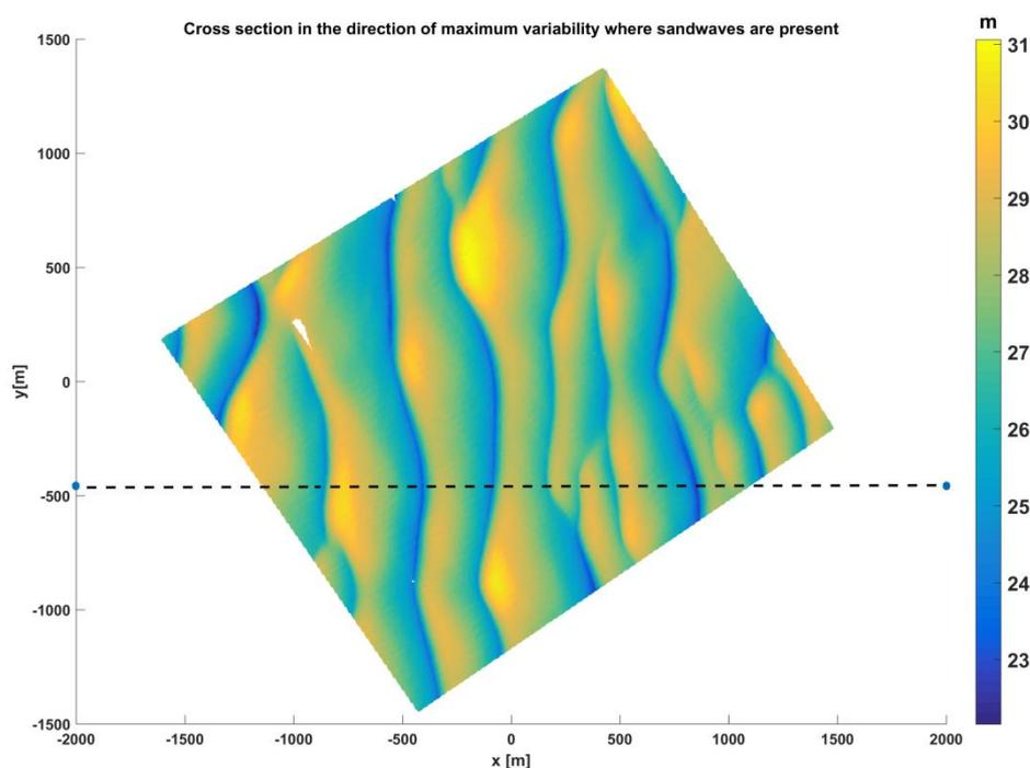
Figure 1: Example of a MBES dataset where sand waves are present showing the cross section taken in the direction of maximum variability.
